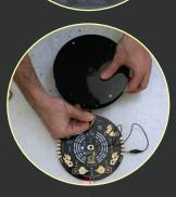
2. CONNECT TO YOUR BIY BOARD TO THE SERIAL PORT OF THE ROBOT
